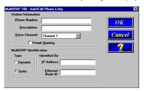
In the **Station Information** group, enter the unique phone number of the local device connected to Channel 1 in the **Phone Number** box. For example phone number 101.
