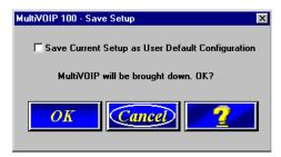
19. Select the **Save Current Setup as User Default Configuration** check box and click **OK**. After the setup is written to the MultiVOIP, the unit reboots.
